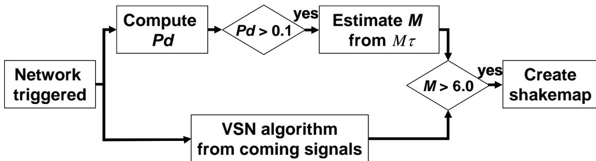
**Figure 4.** Flow chart of the algorithm designed for EEW system in this study. In this design, the VSN and P-wave method operate in parallel.
